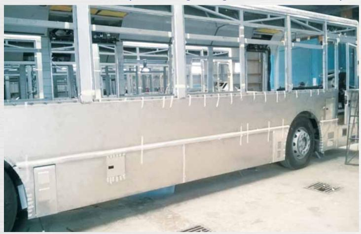
The use of stainless steel in public transport system has been widely accepted worldwide on account of its sterling features providing safety, aesthetics, light weight, fuel efficient and sustainable option. Today, stainless steel is increasingly being used in the construction of medium and long distance buses in the structural parts as well as side paneling, floor and luggage compartments.
